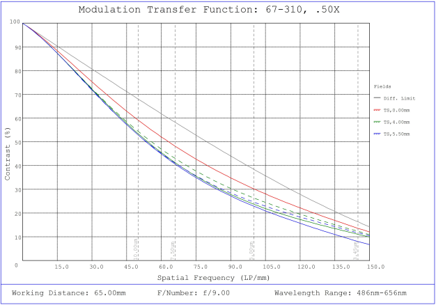
#67-310, 0.5X, 65mm WD, In-Line CompactTL™ Telecentric Lens, Modulated Transfer Function (MTF) Plot, 65mm Working Distance, f9
