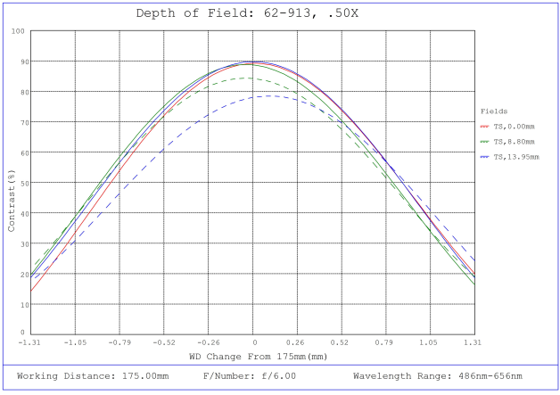
#62-913, 0.5X, 28.7mm M42 x 1.0 (6.56mm) PlatinumTL™ Telecentric Lens, Depth of Field Plot, 175mm Working Distance, f6
