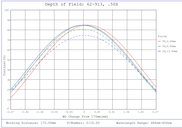
#62-913, 0.5X, 28.7mm M42 x 1.0 (6.56mm) PlatinumTL™ Telecentric Lens, Depth of Field Plot, 175mm Working Distance, f10
