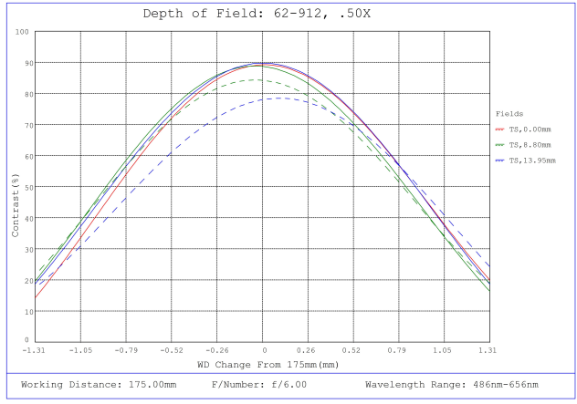
#62-912, 0.5X, 28.7mm F-Mount PlatinumTL™ Telecentric Lens, Depth of Field Plot, 175mm Working Distance, f6
