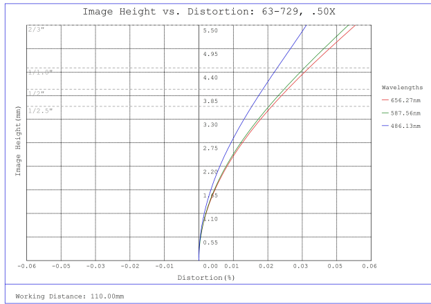
#63-729, 0.5X, 110mm WD CompactTL™ Telecentric Lens, Distortion Plot
