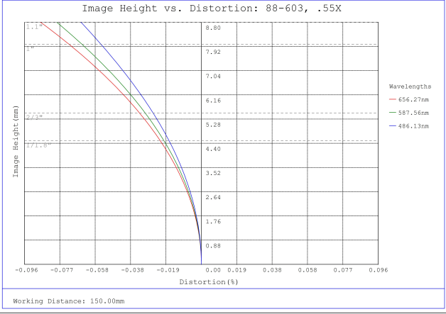
#88-603, 0.55X CobaltTL Telecentric Lens, Distortion Plot
