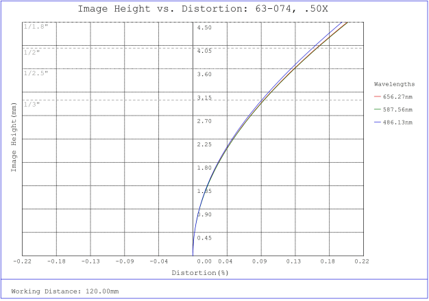
#63-074, 0.50X SilverTL™ Telecentric Lens, Distortion Plot
