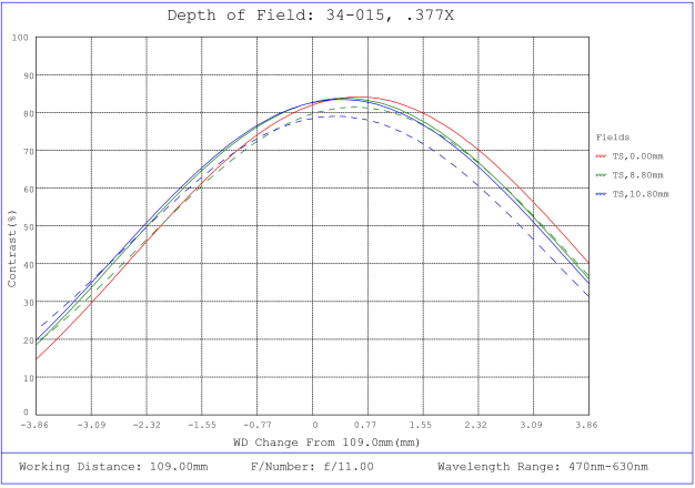
#34-015, 0.377X, 4/3" C-Mount TitanTL® Telecentric Lens, Depth of Field Plot, 109mm Working Distance, f11
