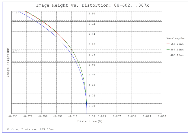
#88-602, 0.367X Cobalt TL Telecentric Lens, Distortion Plot
