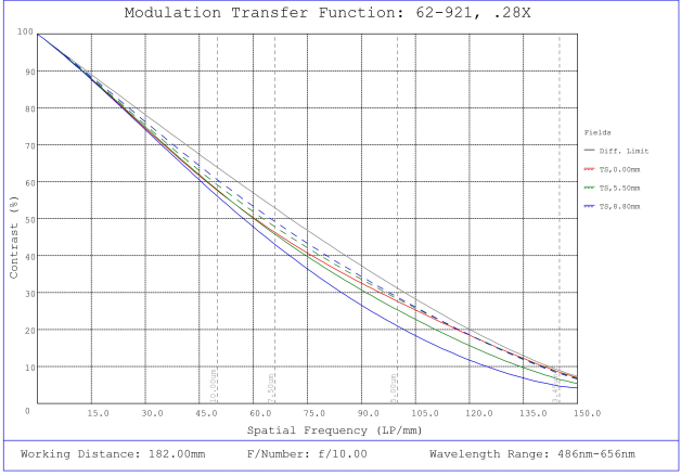
#62-921, 0.28X CobaltTL Telecentric Lens, Modulated Transfer Function (MTF) Plot, 182mm Working Distance, f10
