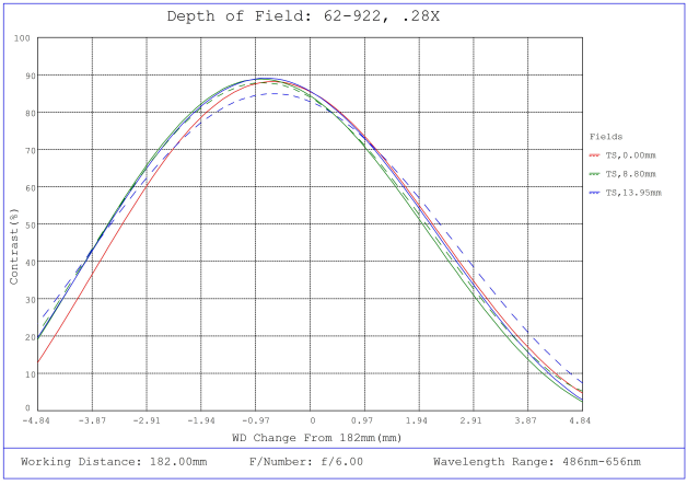
#62-922, 0.28X, 28.7mm F-Mount PlatinumTL™ Telecentric Lens, Depth of Field Plot, 182mm Working Distance, f6
