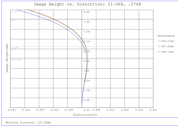
#21-068, 0.274X Cobalt TL Telecentric Lens, Distortion Plot
