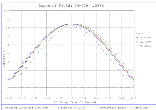
#34-010, 0.268X, 1" C-Mount TitanTL® Telecentric Lens, Depth of Field Plot, 110mm Working Distance, f11
