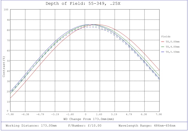
#55-349, 0.25X 2/3" GoldTL™ Telecentric Lens, Depth of Field Plot, 173mm Working Distance, f10
