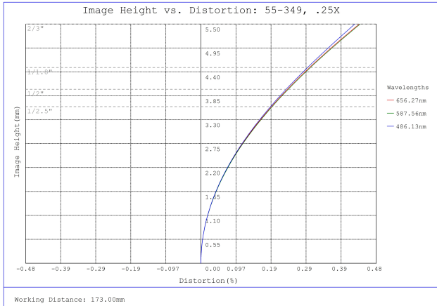
#55-349, 0.25X 2/3" GoldTL™ Telecentric Lens, Distortion Plot
