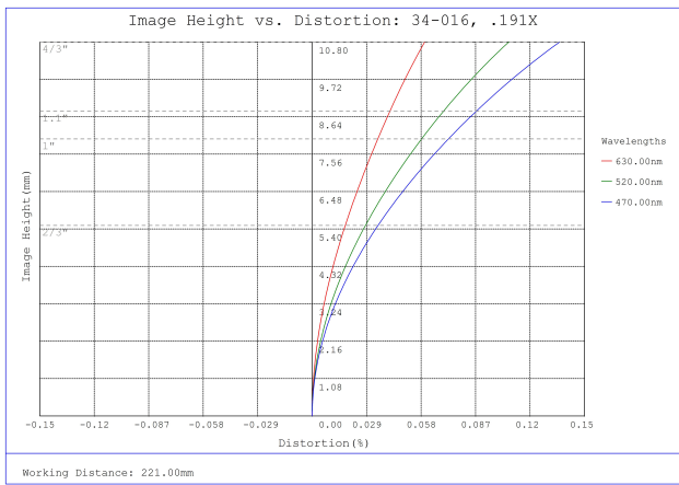
#34-016, 0.191X, 4/3" C-Mount TitanTL® Telecentric Lens, Distortion Plot
