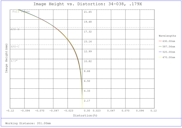
#34-038, 0.179X, 35mm M58 x 0.75 TitanTL® Telecentric Lens, Distortion Plot
