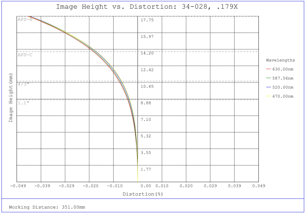
#34-028, 0.179X, 35mm M42 x 1.0 TitanTL® Telecentric Lens, Distortion Plot
