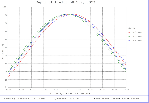
#58-259, 0.09X ½" GoldTL™ Telecentric Lens, Depth of Field Plot, 157mm Working Distance, f6
