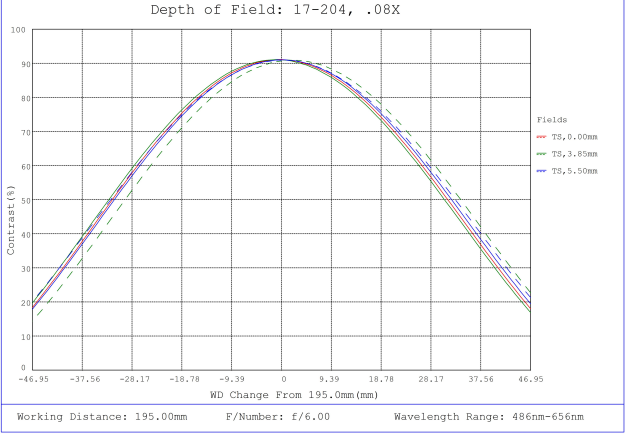
#17-204, 0.08X GoldTL™ Telecentric Lens (Mount Included), Depth of Field Plot, 195mm Working Distance, f6
