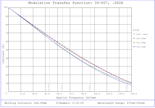
#34-007, 0.060X, 2/3" C-Mount TitanTL® Telecentric Lens, Modulated Transfer Function (MTF) Plot, 284mm Working Distance, f10
