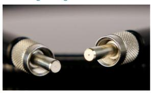
Due to their high numerical aperture of 0.5, our hard polymer-clad step-index multimode fibers are particularly suitable for our light sources and get the maximum optical power from them. They have excellent transmission in the wavelength range 300 - 1200nm. The fibers are equipped with a SMA-905 connector and a heat sink on both sides. A flexible protective sleeve made of stainless steel with a black plastic sheath protects the fiber from damage.
