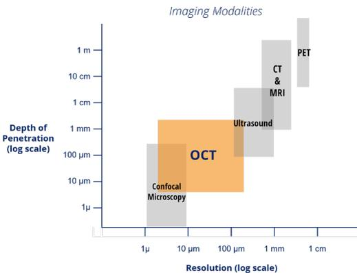
Both are non-invasive imaging techniques used to create both 2D and 3D images of, often biological, samples. However, while ultrasound may resolve centimeters of depth at millimeter resolution, OCT resolves a few millimeters at micron resolution.
