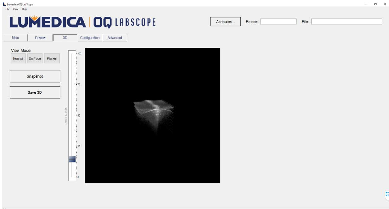
After a volume scan has been captured, the rendering will be available to save from the 3D tab. Rotate the rendering by clicking and dragging across the image. Use the mouse scroll wheel to zoom in and out of the image.
