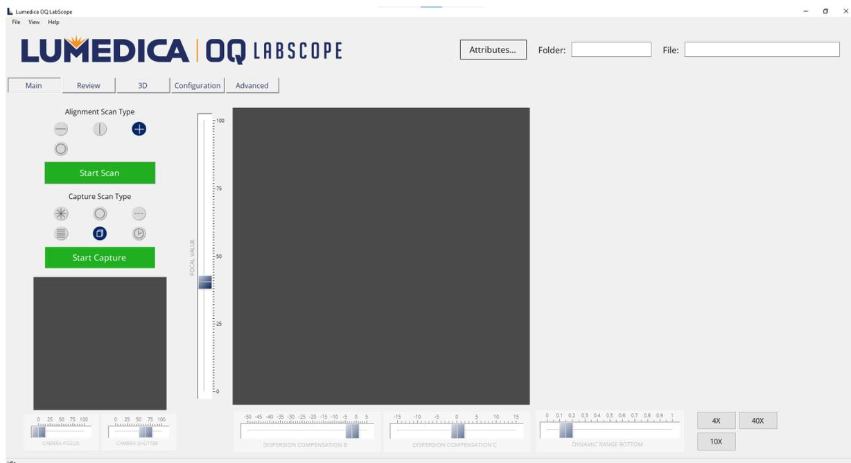
This is the main tab of the OQ LabScope 3.0. As indicated by the text in the bottom left corner, the scanner is in "idle" which means the scanner was successfully initialized and the system is ready to begin scanning.
