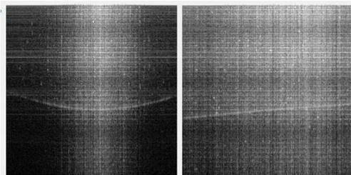
*The image above is the "flipped conjugate" of tape. This image indicates your sample is too close to the scanner.*
