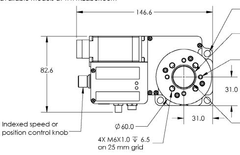
Mounting holes for \_M6 or [1/4"-20] screws at 50 mm [2"] grid spaced around centre of rotation
