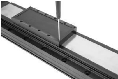
Remove the carriage ramps by removing their screws.
