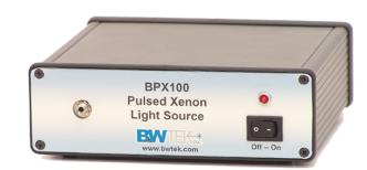
The BPX100 is a compact 5 watt Xenon flash lamp module complete with an internal power supply and trigger circuitry. It is similar to all other arc lamps in that optical radiation is produced by passing an electrical current through a gas. Xenon is the most efficient gas for the BPX100 and produces both continuous and line spectra. Current is supplied by a charged capacitor capable of discharging large
