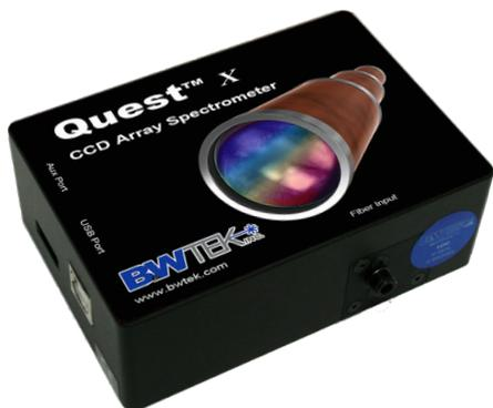
The Quest™ X is a linear CCD array spectrometer optimized for UV and NIR performance using a low stray light optical bench. It features a 2048 element detector, built-in 16-bit digitizer, USB 2.0 interface with a >2.0 MHz readout speed, and external trigger. The Quest™ X is temperature compensated, which greatly reduces the thermal drift to ~15 counts/°C. This gives improved stability by decreasing baseline drift and sustaining the dynamic range.
