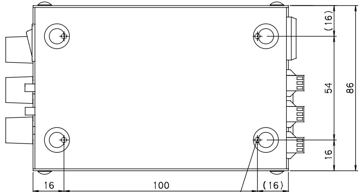
4-M3(screw hole for securing)
