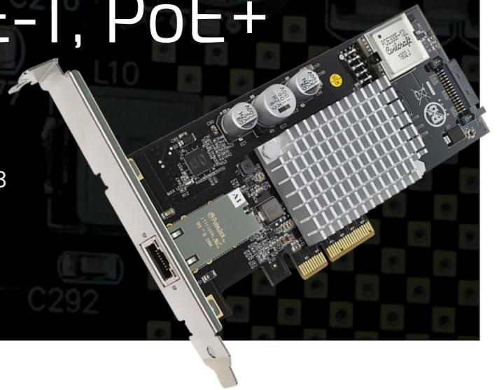
PCIe-POE1-MG2 supports a single 10GBASE-T Ethernet channels in compliance with the IEEE 802.3an and 802.3bz standard, as well as 5.0 Gbps and 2.5 Gbps Ethernet speeds over standard Cat 5e and Cat 6 copper cables. This card is a high-performance PCIe 3.0 Multi-Gig 10GBASE-T/ 5GBASE-T/ 2.5GBASE-T/ 1000BASE-T/ 100BASE-TX Ethernet adapter. It incorporates Aquantia's AQrate PHY technology to deliver 1 GbE and 2.5 GbE network connectivity speeds over 100 m with zero change required for legacy cabling.
