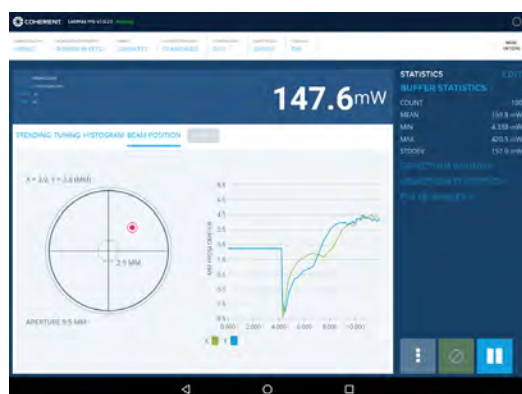
Beam Position with LM-model Thermopiles
