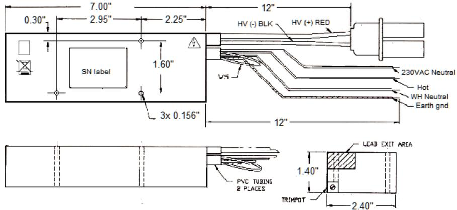
**Figure 14- Module 380T Series Power Supply Dimensions**
