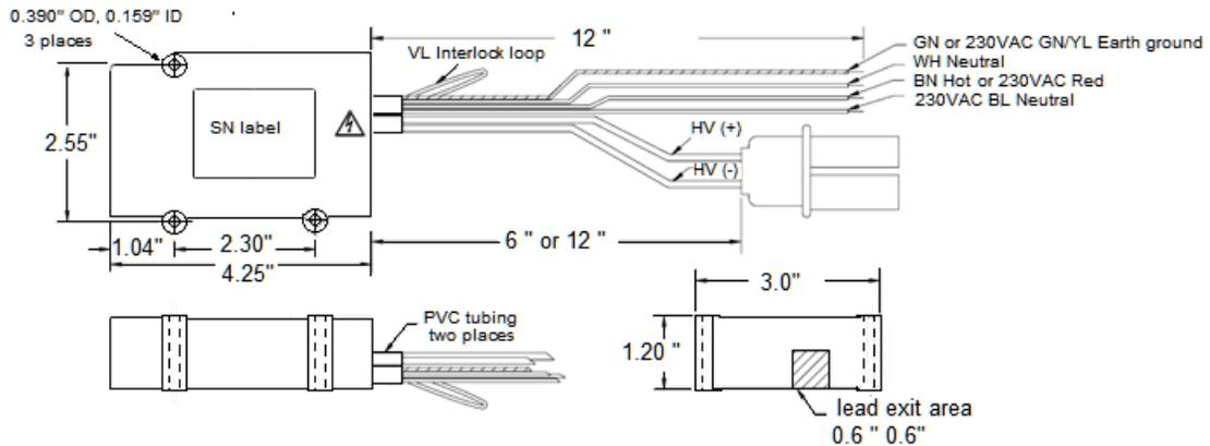
**Figure 13- Module 314T Series Power Supply Dimensions**
