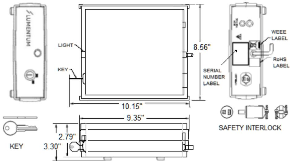
**Fig. 11- Large Model 1200 Series Power Supply Dimensions.**
