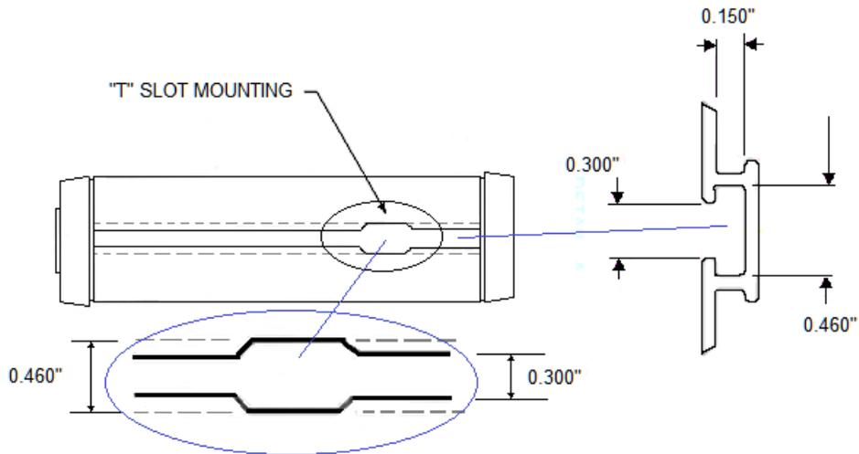
**Figure 6: Model 1500 Series Bottom Plate Slot Mount**
