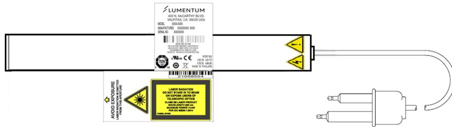
**Figure 1: Placement of Safety Labels on 1100 Lasers**
