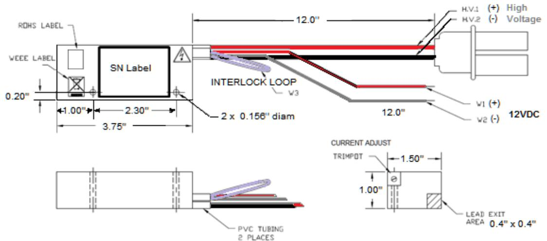
**Figure 12- Module 101T Series Power Supply Dimensions**
