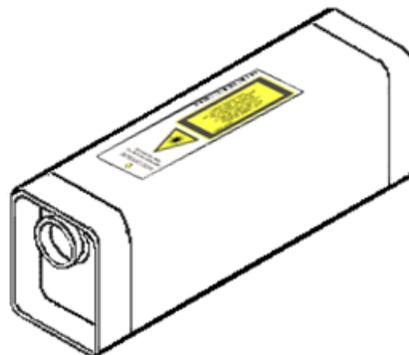
**Figure 2: Placement of Safety Labels on 1500s Laser**
