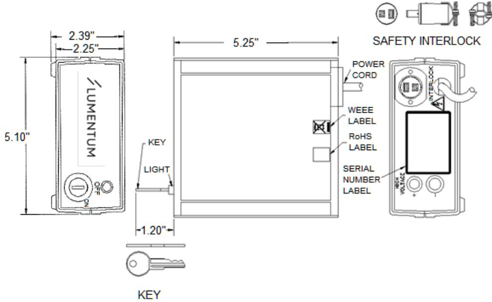
**Fig. 10- Small Model 1200 Series Power Supply Dimensions.**
