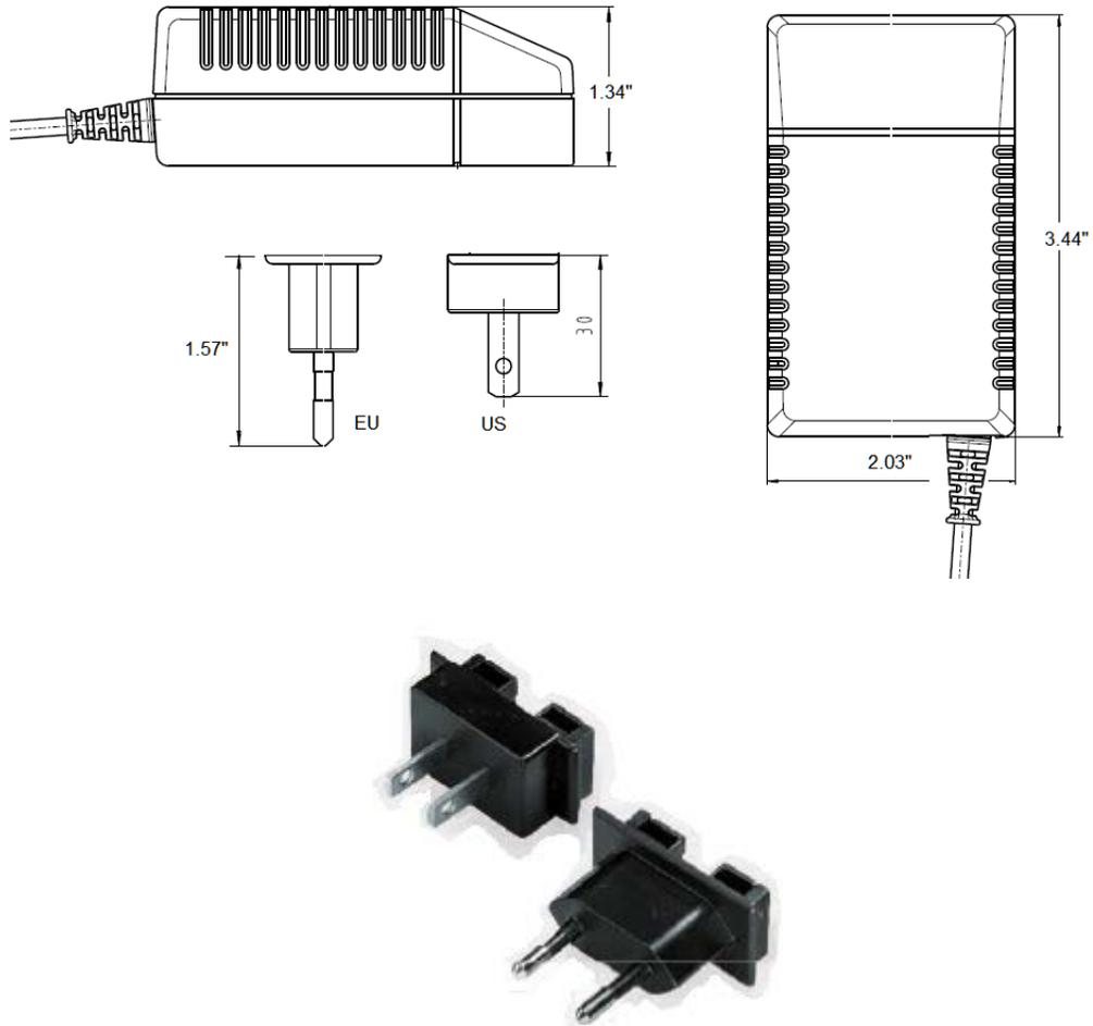
**Figure 7: Model 1500 Series Power Supply Dimensions**
