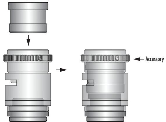
4. Adjust Locknut position until desired focus is achieved. See section on Working Distance and Field of View below to find Locknut positions. Tighten Nylon Tip Set Screw into place for a focal position that can later be readjusted—the nylon tip will protect the threads. To set focal position permanently, install the socket head screws. Do not overtighten screws.
