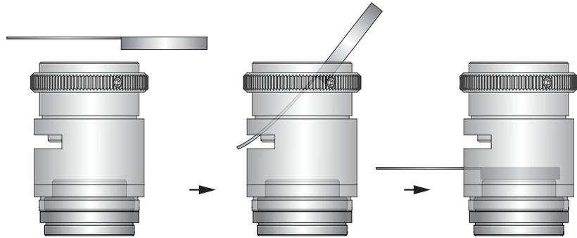
3. Using a spanner wrench, thread the bottom of Rear Assembly into the top of Main Housing until it is flat against the accessory, hand tightening torque or about 2.5-5kgf\*cm. If using a Liquid Lens, hold the Liquid Lens in place while tightening the Rear Assembly into Main Housing by inserting a paperclip into one of the holes to the side of the Liquid Lens Holder. (Optional: spanner wrench #35-029 can be used)
