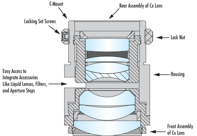
**Figure 1:** 35mm Cx lens without the required accessory.
