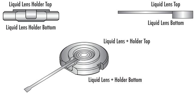
**Warning: Liquid Lens ribbon is fragile. Use caution when assembling unit and during handling.**
