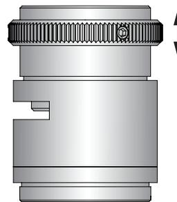
5. Thread entire assembly into C-Mount camera from the top of Rear Assembly until the top of the Locknut is flush against the camera C-Mount.
