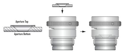
\*Appearance of Aperture for each focal length and f/stop may vary slightly, but the side of the aperture with the larger diameter hole is always the top.
