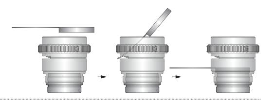
3. Using a spanner wrench, thread the bottom of Rear Assembly into the top of Main Housing until it is flat against the accessory, hand tightening torque or about 2.5-5kgf\*cm. If using a Liquid Lens, hold the Liquid Lens in place while tightening the Rear Assembly into Main Housing by inserting a paperclip into one of the holes to the side of the Liquid Lens Holder. (Optional: spanner wrench #35-029 can be used)
