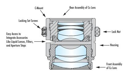
Figure 1: 25mm Cx lens without the required accessory.
