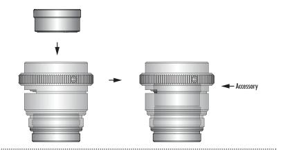
4. Adjust Locknut position until desired focus is achieved. See section on Working Distance and Field of View below to find Locknut positions. Tighten Nylon Tip Set Screw into place for a focal position that can later be readjusted-the nylon tip will protect the threads. To set focal position permanently, install the socket head screws. Do not overtighten screws.
