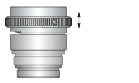
5. Thread entire assembly into C-Mount camera from the top of Rear Assembly until the top of the Locknut is flush against the camera C-Mount.
