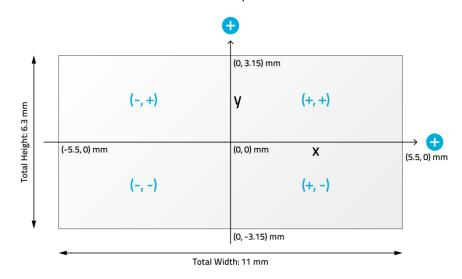
Figure 5-3 Fixed Coordinates System for the Sensor
