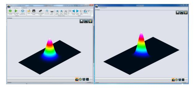
Figure 4-2 The PC-BeamPro Interface With and Without the Main Controls Ribbon
