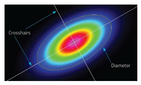
Figure 6-3 2D Display Showing Crosshairs and Diameter Positions
