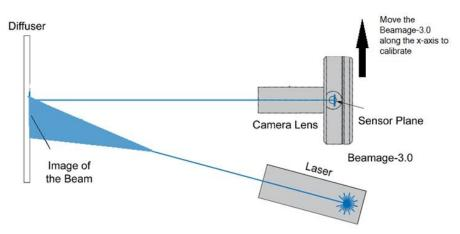
Figure 5-17 - Camera Lens Calibration Moving Direction
