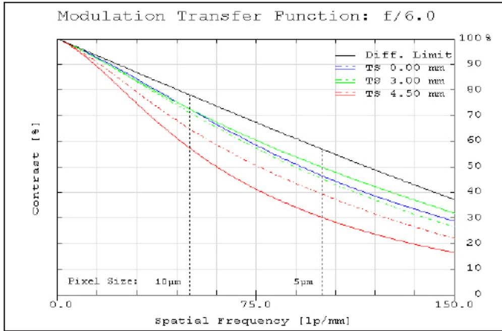
**Figure 3:** Image space polychromatic diffraction FFT Modulation Transfer Function (MTF) for  $\lambda = 486\text{nm}$  to  $656\text{nm}$ . Included are Tangential and Sagittal values for field points on center, at 70% of full field and at the maximum sensor format. Solid black line indicates diffraction limit determined by  $f/\#$ -defined aperture. Frequencies corresponding to the Nyquist resolution limit of pixel sizes are indicated.
