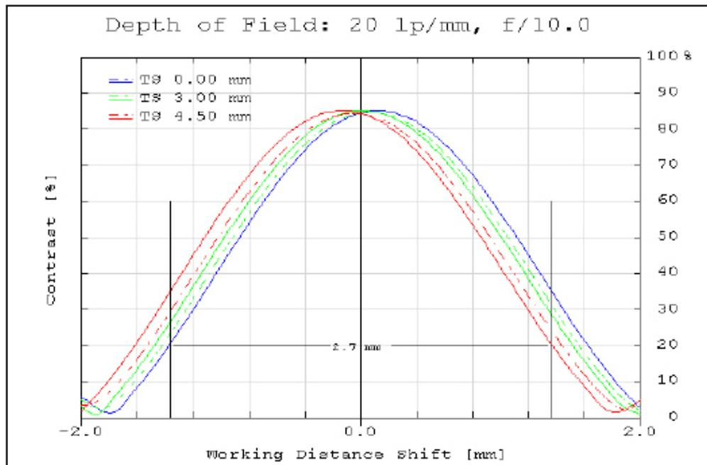
**Figure 6:** Polychromatic diffraction through-focus MTF at 20 linepairs/mm (image space). The depth of field at the maximum sensor format for the plotted frequency and  $f/\#$  at 20% contrast is indicated by the measurement bars.
