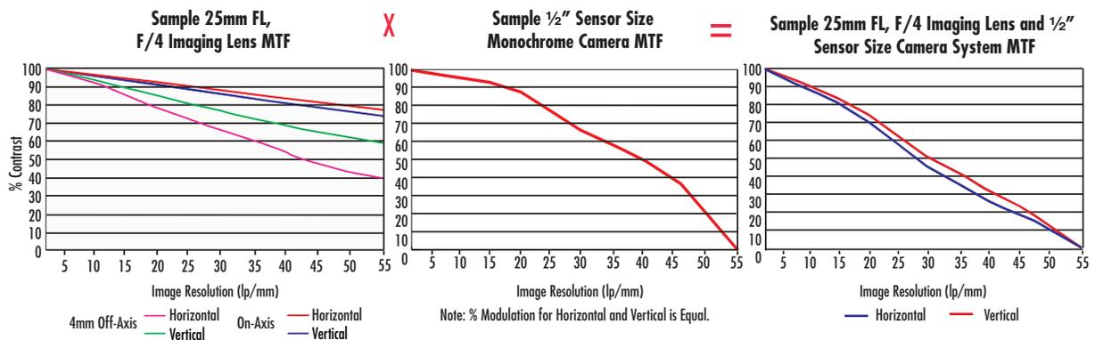
Figure 4: System MTF is the Product of the MTF of Each Individual Component
