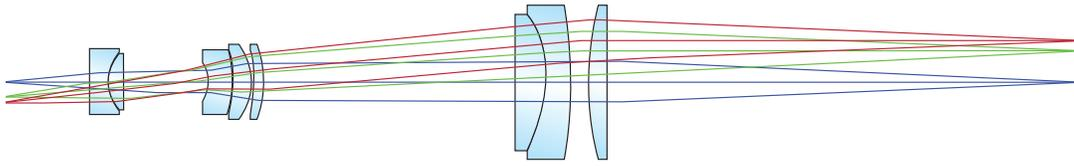
Figure 2: 0.5X Image-Space Telecentric Lens (Note the Parallel Chief Rays in Image Space)
