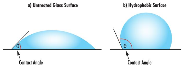
**Figure 2.** Two water droplets on horizontal glass surface. a) There is a smaller contact angle on the untreated surface, indicating higher surface tension. b) There is a larger contact angle on the hydrophobic surface, indicating lower surface tension.
