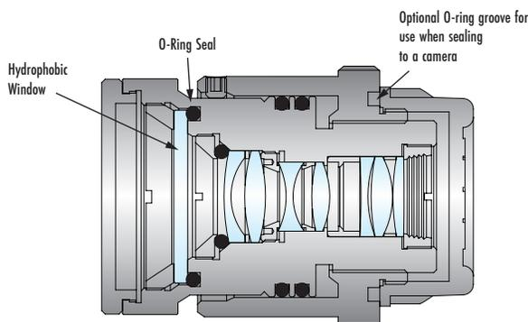
**Figure 1.** Internal schematic of a Cw Series Lens.
